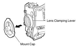
2 Align the indentation at the top center of the lens mount with the center mark of the lens and mount the lens.
